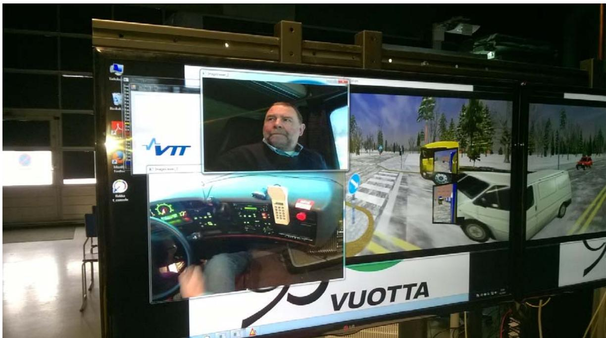
Control panel of TTS simulator during piloting
